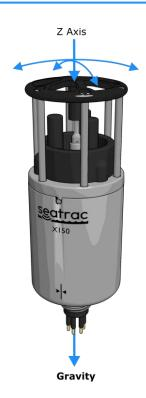
Finally, once you are happy with that all 6 limit values have been obtained, click the "Calculate" button (under the Accelerometer group) to compute the calibration and store the values into permanent Flash memory. This completes the Accelerometer calibration for pitch and roll.
